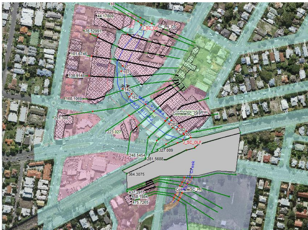
Figure A6: Geometric plan view – Stormwater drainage network at Colmslie shopping Centre
