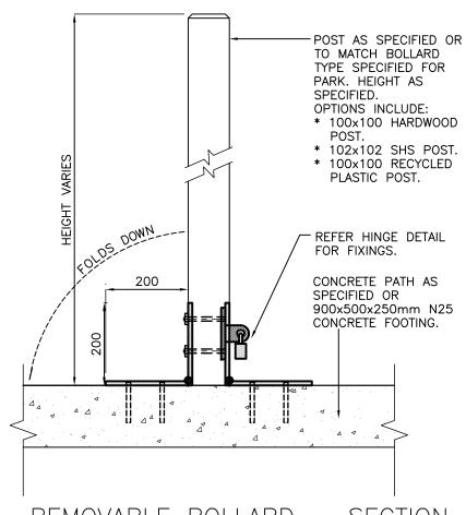
REMOVABLE BOLLARD — SECTION SCALE: 1:10
