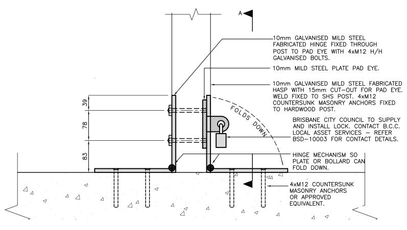
REMOVABLE BOLLARD — HINGE DETAIL SCALE: 1:5
