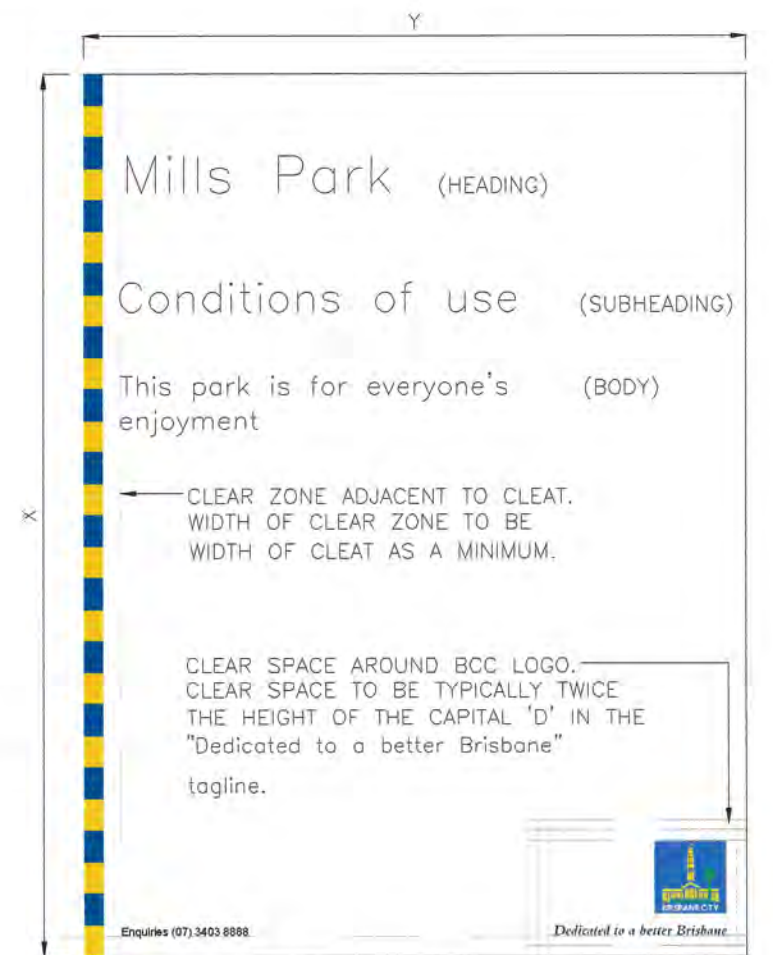
TYPICAL GRAPHIC LAYOUT Enquires (07) 3403 8888 PORTRAIT ORIENTATION CLEAT (SIZE AS PER TABLE) REFER TO TABLE BELOW FOR TEXT STYLE SIZES RELATIVE TO SIGN SIZE. CLEAT UNIT DETAIL
