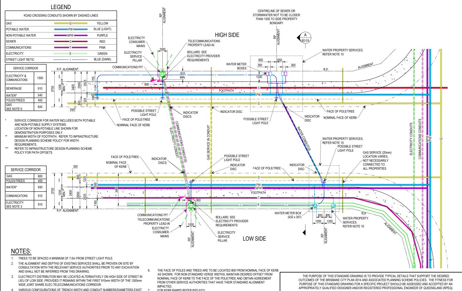
FOR BOTH ELECTRICITY AND COMMON TRENCH ARRANGEMENTS WITH COMMUNICATIONS. REFER ELECTRICITY AUTHORITIES STANDARD DRAWINGS. PREFERABLY COMMUNICATIONS CONDUITS SHOULD BE INSTALLED IN SHARED TRENCHES
