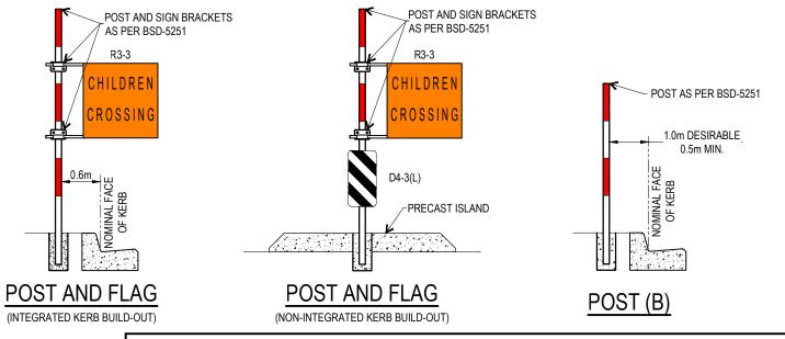
THE PURPOSE OF THIS STANDARD DRAWING IS TO PROVIDE TYPICAL DETAILS THAT SUPPORT THE DESIRED OUTCOMES OF THE BRISBANE CITY PLAN 2014 AND ASSOCIATED PLANNING SCHEME POLICIES. THE FITNESS FOR PURPOSE OF THIS STANDARD DRAWING FOR A SPECIFIC PROJECT SHOULD BE ASSESSED AND ACCEPTED BY AN APPROPRIATELY QUALIFIED DESIGNER AND/OR REGISTERED PROFESSIONAL ENGINEER OF QUEENSLAND (RPEQ).
