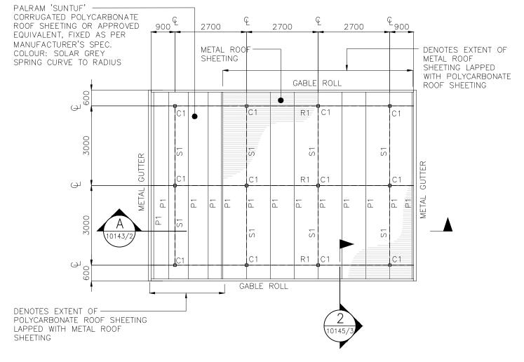
ROOF FRAMING PLAN SCALE 1:100
