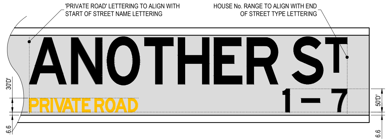
PRIVATE ROAD STREET NAME PLATE (COUNCIL LOGO, CLEAT AND STREET NAME LETTERING AS PER GENERAL STREET NAME PLATE DETAILS)
