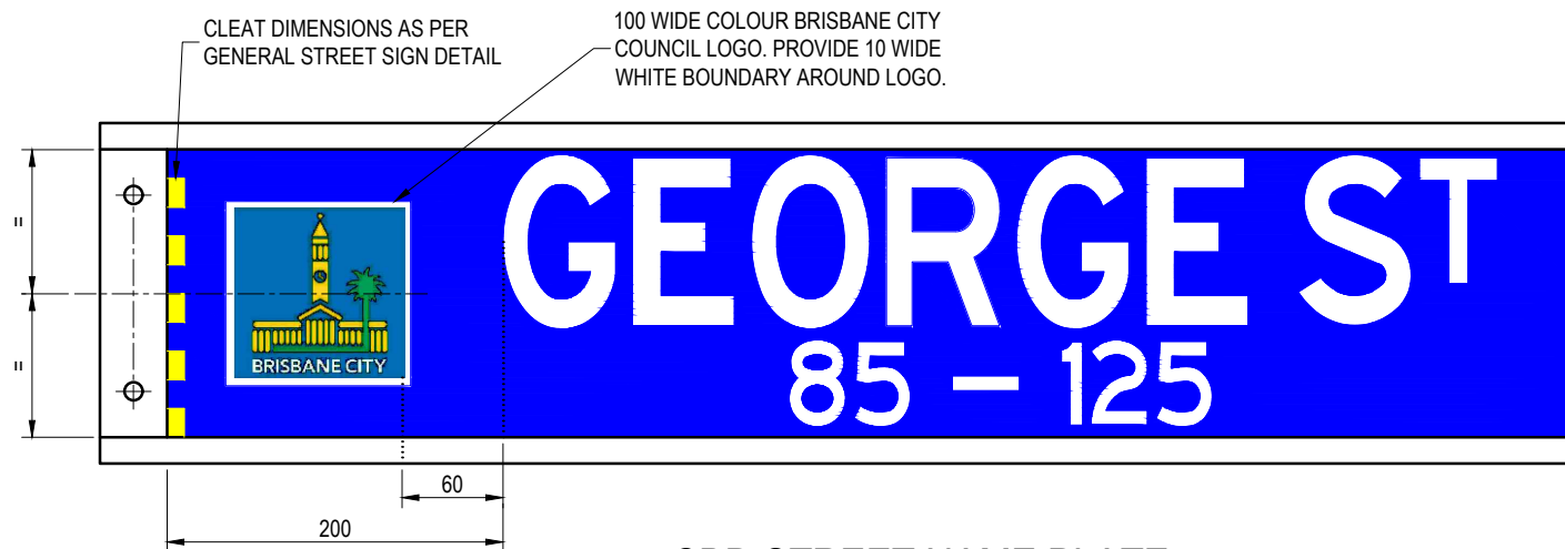
CBD STREET NAME PLATE (STREET NAME LETTERING AS PER GENERAL STREET NAME PLATE)
