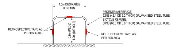
HANDRAILS TO BE GALVANISED TUBE ROLLFORMED FROM ONE PIECE OF PIPE IN ACCORDANCE WITH AS1163
