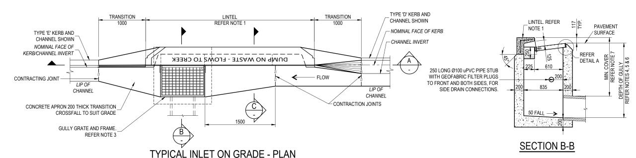
NOTE: FOR SAG GULLY, APRON TO EXTEND TO END OF LINTEL AND GULLY TO BE LOCATED IN CENTRE OF LINTEL.
